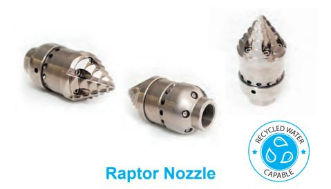
The Raptor Nozzle is a powerful nozzle capable of removing heavy obstructions caused by roots, grease, or any other solid organic material quickly. Its tempered stainless steel drill head is turbine-driven and spins in the range of 6000 and 12000 rpm, depending on water flow and pressure. The Raptor Nozzle succeeds where standard hydromechanic tools fail!
