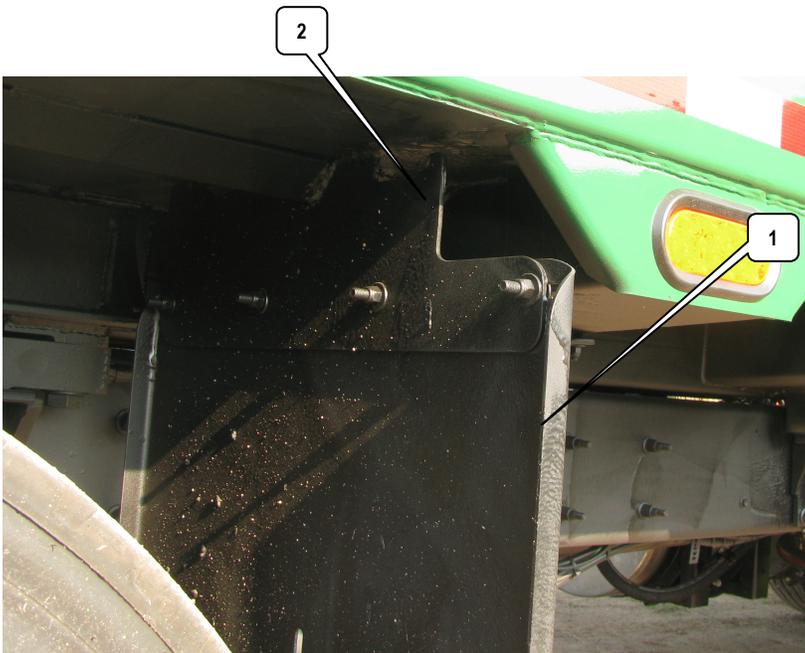
These "ahead of the tandem" STEEL Mudflaps are OPTIONAL..but **every** DMSLH (Demolition) has these STEEL Mudflaps as "**Standard**" to DMSLH's "package" <Note: Complete Pair of Steel Mudfaps KIT BOM is 0120211>
