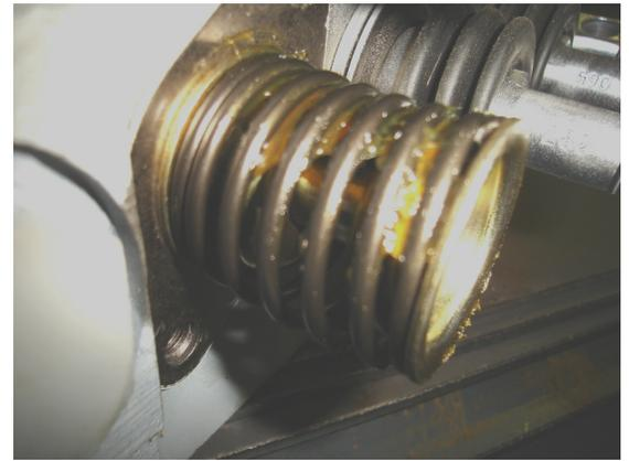
**NOTE:** Assure the correct "Orientation" of items 1 & 2 as imaged here (Assure CORRECT orientation...or seal system will "fail")
