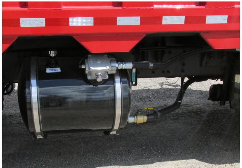
Frame-Mounted Oil Tank... aka.. "FRAME TANK"
