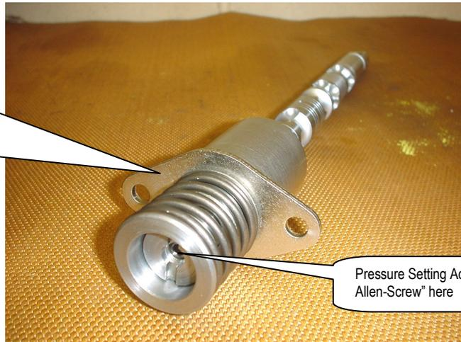
Pressure Setting Adjustment is a Allen-Screw here
