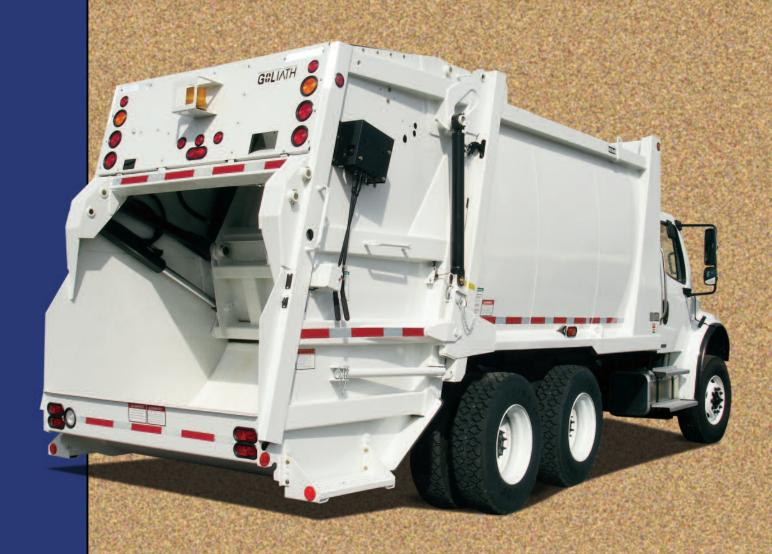
Simple, Lightweight Design for High Compaction Reliability
