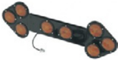
△ 8-Lamp Arrow Board Kit A120394 (Incandescent) 12V Lamp, includes controller and 55' of cable.
