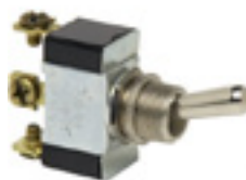
△ Toggle Switch A120861-2 SPDT, Mom. On - Off - Mom. On. 3 screw terminals. 25A@12VDC. Side Panel, Boom Controls, Throttle Control (units with ICM control) Side Panel, Rear Door (tailgate), Side Panel, Rear Door Locks.
